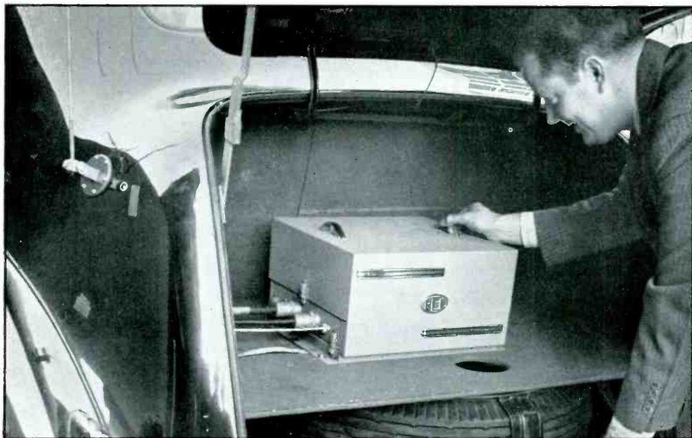
FIG. 1. REL TRANSMITTER, RECEIVER, AND POWER SUPPLY ARE CONTAINED IN A SINGLE DUST-TIGHT UNIT
