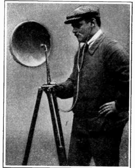
The new infra-red ray receiver in use
