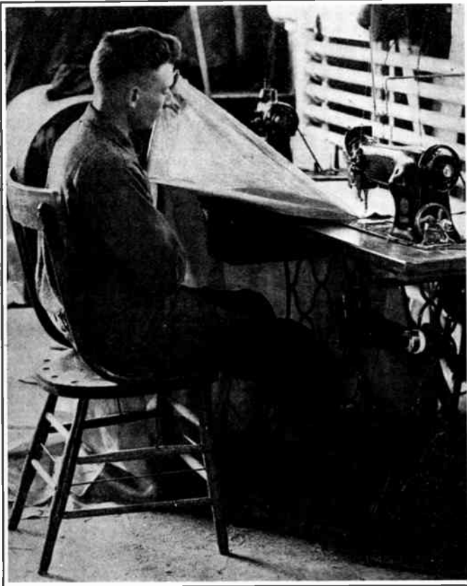
Stitching pieces of cloth together to form a bag to be used as airplane wing covering
