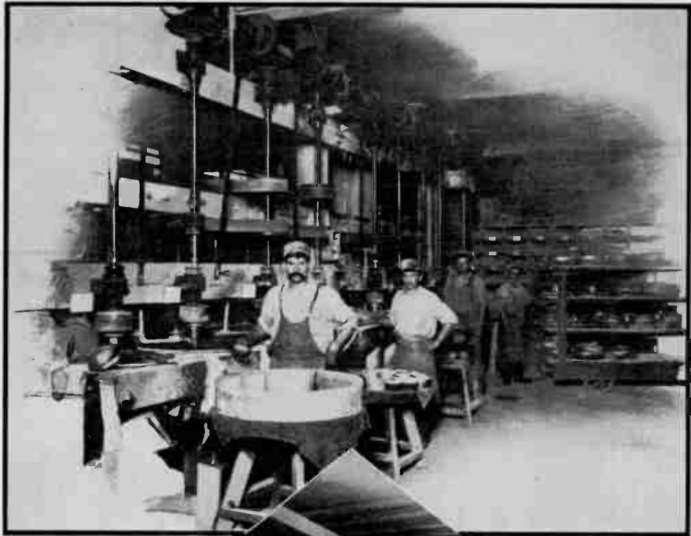
Puttling Carborundum wheels. The mixture of grains and bond are placed in the large forms shown
