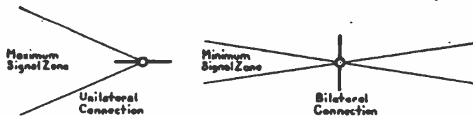
Fig. 12. By listening in both ways, the transmitter can be located accurately
