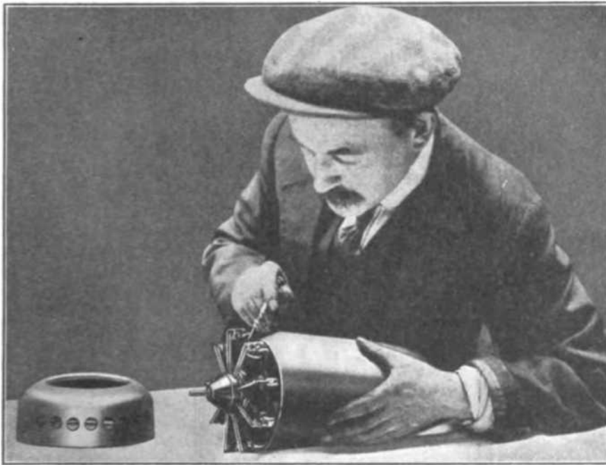
Expert model maker at work on miniature reproduction of nine cylinder rotary airplane motor mounted at front end of nacelle for twin-motored biplane
