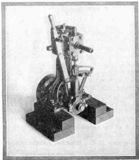
Model of a steam speed boat engine with reversing gear.
