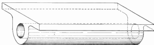
Fig. 25. Appearance of casting showing cored hole.
