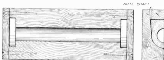
Fig. 24. Plan and end view of half core box. Must be made so that half core may fit together.
