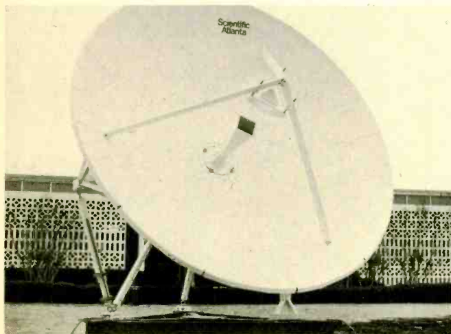
Fig. 9. The parabolic dish reflector gives the highest gain and directivity of any antenna system now in use. It traps nearly all the radio energy which strikes it, and concentrates it to give maximum results. A small dipole or cavity is at the dish's center.
