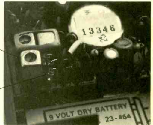
Fig. 2. The discriminator transformer, shown here, has several glass diodes beside it. These take audio from the IF stage.
