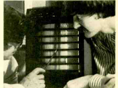
Scientists study a series of spectra showing the progress of a chemical reaction in which the compound methyl isocyanide undergoes an explosive rearrangement of its molecular structure. A new laser technique permits these spectral "snapshots" to be made in a few nanoseconds, which is a lot faster than a Brownie!
