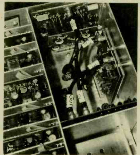
This is the final amplifier circuitry. The RF power transistors are hidden from view. Circle number 1 on reader service card.
