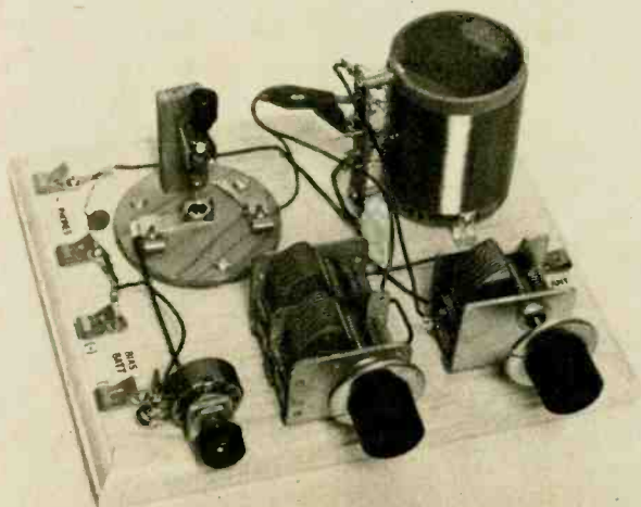
Grandpa's Whisker is a nostalgic look back at the days when a ship's radio lifeline to shore was dependent on no more than a coil, a battery, a catwhisker, and carborundum.
