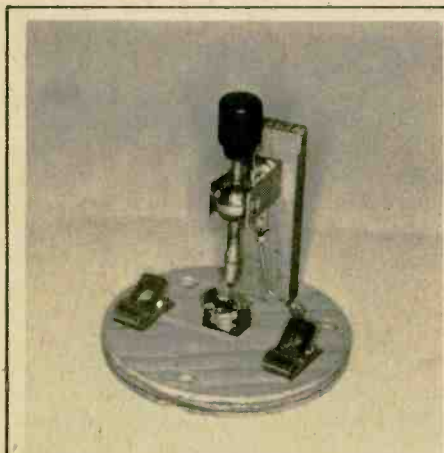
Most of the crystal detector assemblies you can turn up will be of the horizontal type. You will need a heavier pressure for the carborundum crystal, so convert the assemblage to a vertical format. None of the dimensions shown are all that critical.
