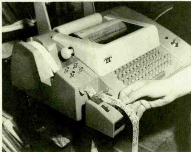
The punch/reader of an ASR-type teletype writer is one of the more common systems. It's very easy to use; just push a button to transmit a signal from the computer and it will punch or read a tape or do both.
