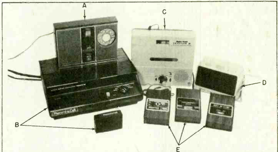
A few of the most popular telephone accessories. A—The Heathkit speakerphone or "hands-free telephone" with built in dialer. B—the Record-A-Call remote control telephone answering machine that can be keyed from a remote location to play messages back over the telephone lines. C—Radio Shack's budget telephone answering machine. D—Radio Shack's low cost speakerphone (no built in dialer). E—An assortment of Telco devices to indicate if your phone is being tapped, to start a recorder each time your phone is used, to provide conference-connection between two telephone lines.
