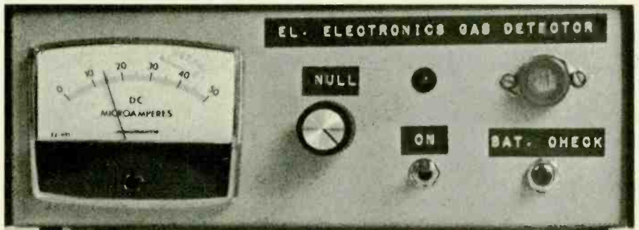
Front view of the Super Sensor shows the positioning of the meter, the null control, and the battery check and off-on switches, as well as the gas detector itself.
