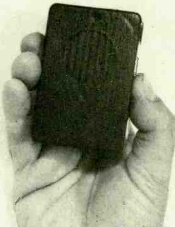
No larger than a pack of cigarettes this tone generator can signal a Record-A-Call to playback all received messages when you phone in. You reset the Record-A-Call with a second tone burst.
