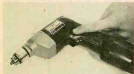
Finger indicates the three-position switch on the handle which permits selection of Forward, Reverse, and Lock functions.
