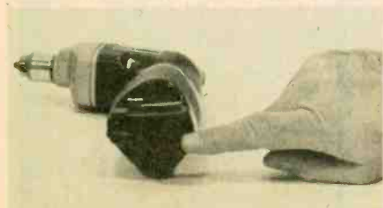
Here we're indicating the small metal tab on bottom of the battery which is pressed, releasing battery from drill body.
