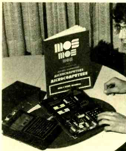
KIM-1 microcomputer can use a recorder as well as other input and/or outputs.
