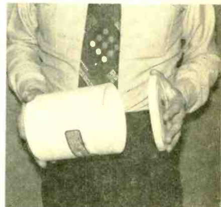
Plastic food container gets cut off near top to secure cover which seals speaker.
