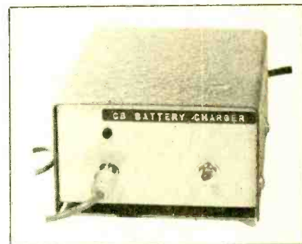
Charger can connect to wide variety of NiCad battery packs using the universal cable described in text.
