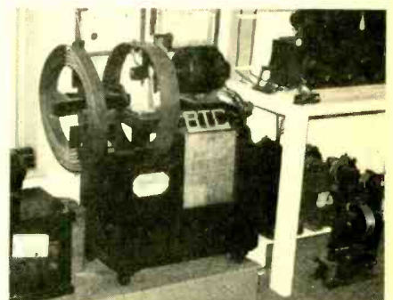
Early transmitter (arc type), one of several on view in the Antique Wireless Association's Museum.
