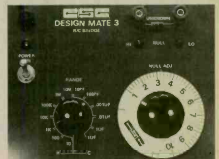
Closeup of Design Mate 3, the R/C bridge shows terminals for unknown capacitor or resistor upper right, large knob and range switch at bottom.
