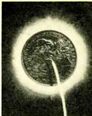
Wire to earth ground is used when Kirlianizing objects other than humans. The corona discharge, as around this silver dollar, is clearly visible in a dark room. A double exposure was used in this camera shot to show the wire and coin surface, and the cumulative effect of prolonged Kirlian discharge.
