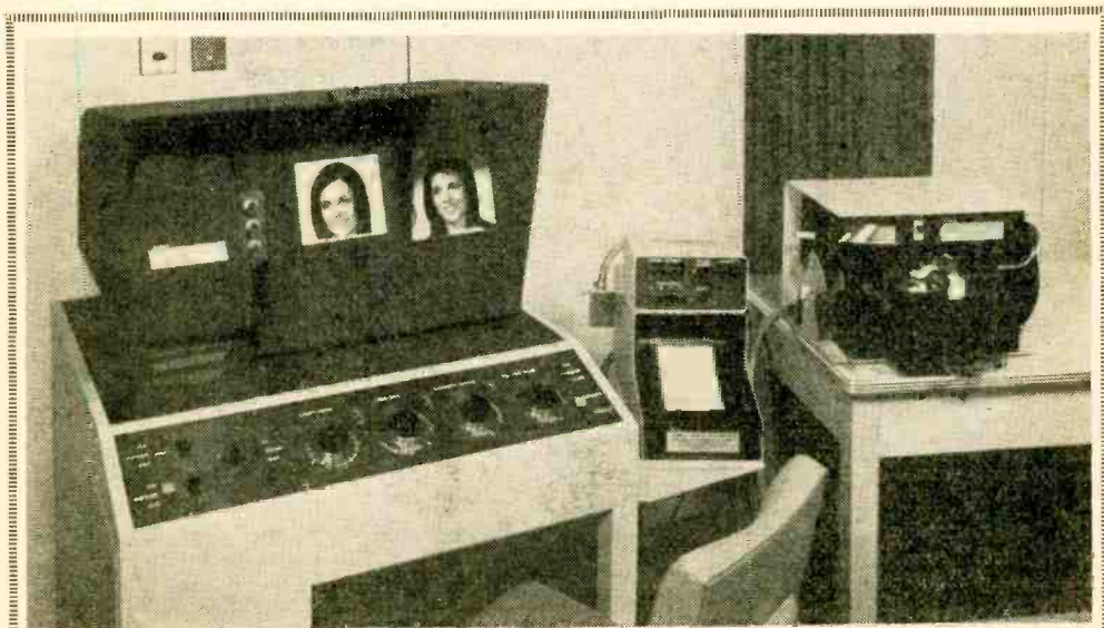
Professional equipment used by color labs includes this Kodak Video Color Negative Analyzer. It uses a 5-in. color TV screen to assist an operator in selecting the correct filter.
