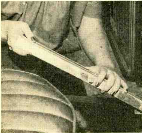
The best way to make a neat installation is to use the car's cable channel just under edge molding located on the driver's side.
