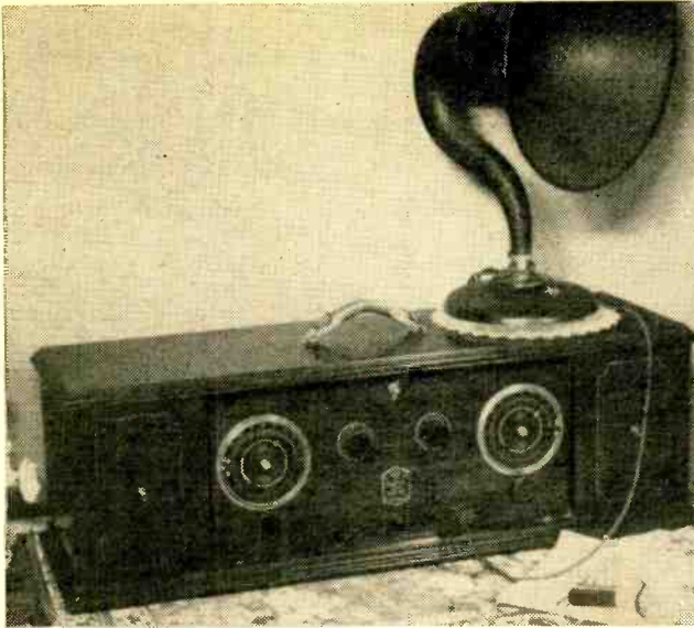
A completely restored superheterodyne receiver, a 1924 Radiola, was the result of the pioneering efforts and developments of Major Edwin Armstrong and his early staff.
