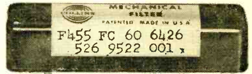
Fig. 7 This is the type of filter used to remove the unwanted sideband from the output signal.
