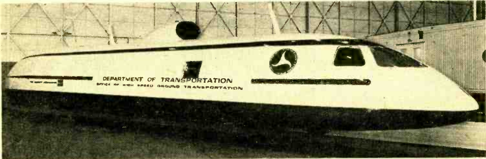
Huge 25-ton test vehicle, capable of traveling 250 mph, is being tested by Garrett Corp., Torrance, Calif. on a low-speed test track.
