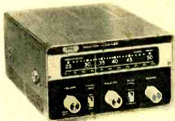
This tunable plus one fixed freq. band receiver operates off 117V AC or 12V DC. Companion hi-band available.
