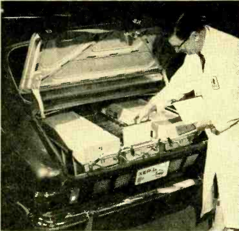
General Motors engineer Harold A. Schulte inserts zinc anodes into one of the six zinc-air batteries which give the experimental XEP car its long range. Developed at the GM Research Laboratories, the electric car can travel about 150 miles at 30 miles per hour.
