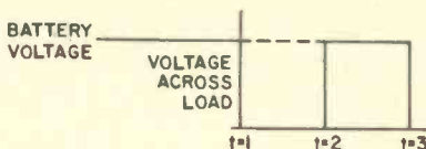
Simple load/battery/switch series setup can be considered square-wave generator. If switch contacts are clean, you'll see pseudo-square waves on your scope as you flip switch rapidly on, then off, again.
