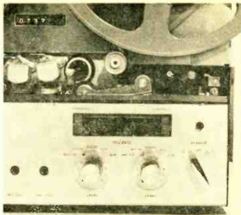
Each input has own individual selector and volume control; power switch simultaneously selects reel size, speed, and equalization.
