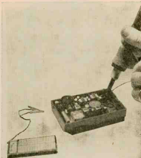
Fig. 13. Careful inspection of the radio can often uncover the problem. When soldering these jobs, use a small low-power iron to avoid damage from excess heat.
