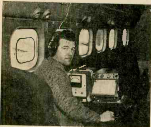
Researcher sits at controls of thermometer that takes water temperatures from high in the sky.
