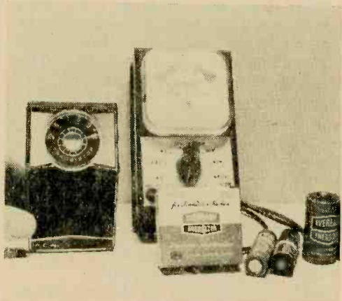
Fig. 9. Weak or corroded batteries are transistor radio's number-one enemy and account for majority of problems. Checking batteries with a good battery checker that tests output voltage under load will locate defective unit.
