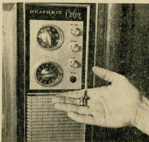
Fig. 2. Lack of color can be caused by incorrect setting of color killer control. On set above, this control is accessible after removing color knob though most sets have control on rear apron.
