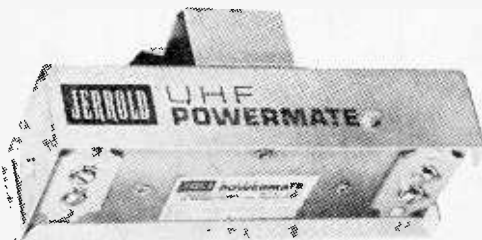
Fig. 11. Wide-band UHF signal boosters are mounted on antenna masts just under the UHF antenna. Tele-Amp unit is shown above and Jerold unit below. Power to units is supplied through TV lead-in wire from indoor supply.
