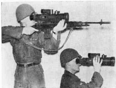
Image intensifier permits soldiers to see in the dark without revealing their presence. Photo shows unit mounted on rifle. Inset shows unit used for spying without rifle.
