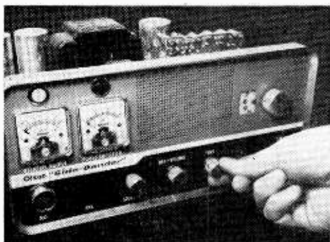
Frequency-synthesis crystal-controlled rig has fine tune for off-frequency incoming signals.
