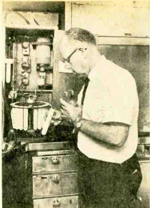
Even test tubes get into the how-bad-is-our-air act during Public Health Service studies. Researcher places air sample and reagent in test tube, then relies on resultant color of tube's contents to determine what foreign gases are present. Below, photo shows part of instrumentation used to measure level of sulfur dioxide in atmosphere. Gas is especially dangerous because of its proclivity to reform into sulfur trioxide and, ultimately, sulfuric acid.
