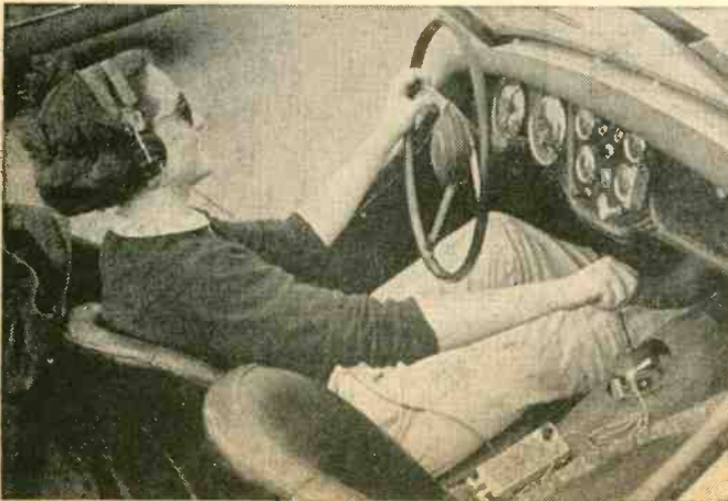
The young lady is checking out her sports-car's transmission with the aid of Super Snoop. Here the transducer is attached right next to the gearshift lever with the C-clamp mount.
