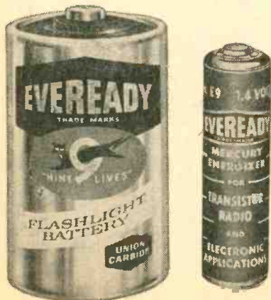
Mercury cell at right is excellent voltage reference source, since open-circuit voltage of 1.3455 remains virtually constant during life of battery. Fresh flashlight cells, though not as accurate, give 1.561 volts.
