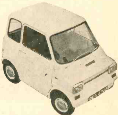
The Ford Comuta (above) is an experimental electric car developed by Ford of Britain's Research Staff. Chassis and batteries of the experimental car are shown in the bottom photo.
