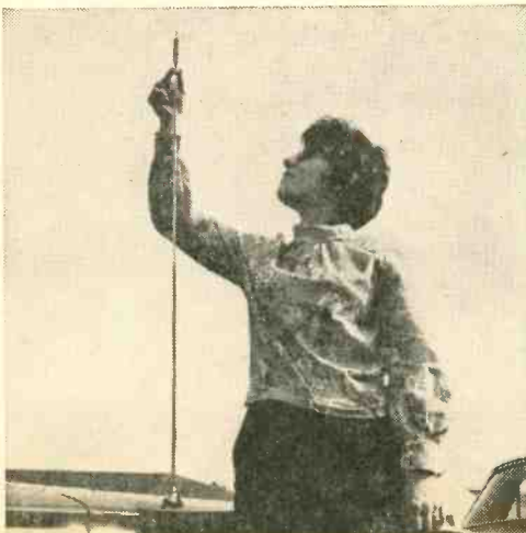
Easiest and most convenient to install of the 6 mobile CB antennas is the CB/AM whip that serves as antenna for both. Unit here is a conversion kit mounting on existing AM antenna.
