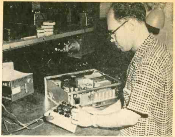
Work in repair shop is generally varied enough to offset possible boredom. Technician above is using grid-emission tester to weed out erratic tubes.
