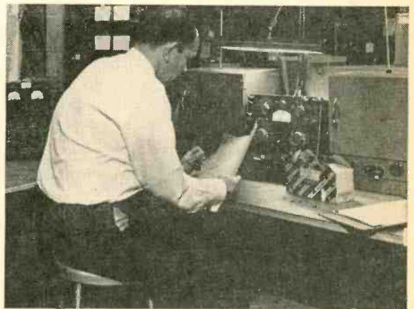
Manufacturing plants generally have well-equipped and well-staffed labs, often with high-precision equipment. This technician is using impedance bridge.
