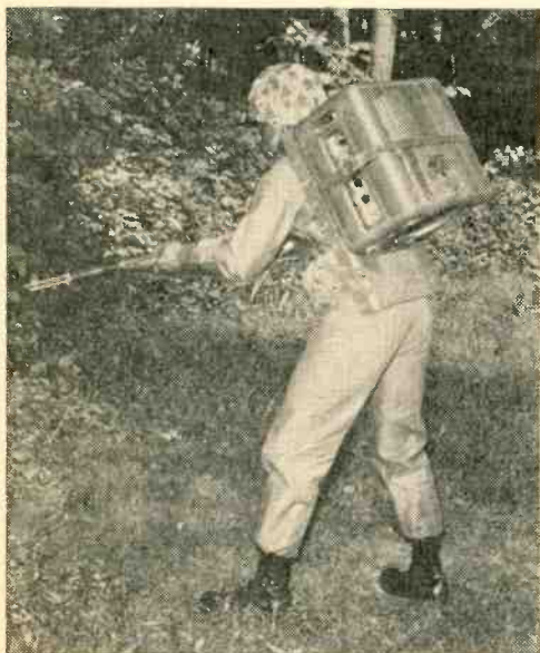
Thermoelectric generator can be easily carried about boy scout style. It weighs only 35 pounds with fuel and is designed to be transported on the soldier's packboard.
