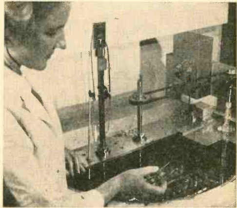
The national practical standard for DC voltage is the average value of a group of very stable saturated standard cells. NBS staff member is making a connection to one of the cells which are kept in an oil bath maintained within a few thousandths of 28° C.
