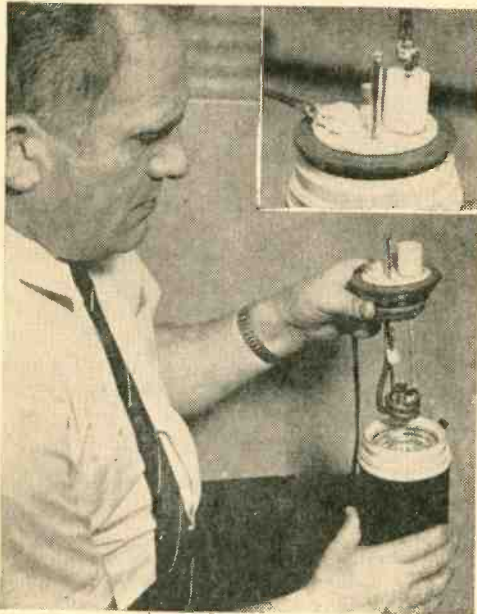
The dewar flask being removed from cryogenic cooler developed at NBS electron devices laboratories. Photo shows gas inlet tube, heat transfer coil, outlet tube, and heater. Device to be cooled is placed within plastic-foam frost shield, which prevents frost accumulation from occurring and interfering with the operation of the device.
