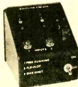
Fig. 1. Demonstration unit has three types of multivibrator circuits easily selected by a front panel 3-position switch.
