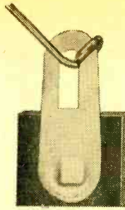
Lead is wrapped around tie-point lug (above) before applying heat to lug (right)—close to wrapped lead end.
