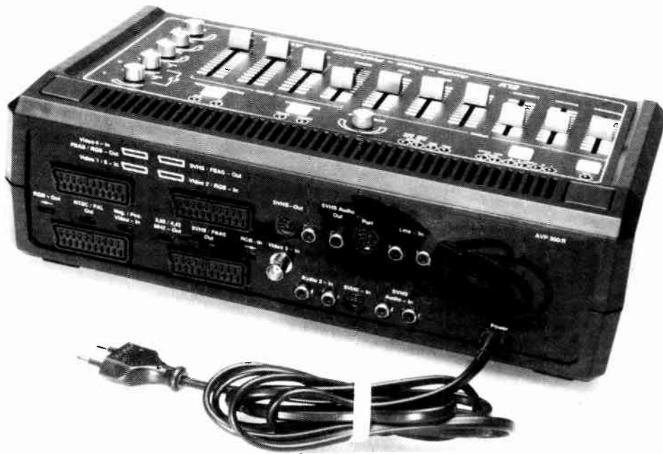
Fig. 2. Rear view of the audio video processor showing the 16 input sockets and the various switches.
