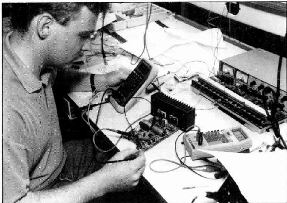
Fig. 3. Initial test on the assembled board.
