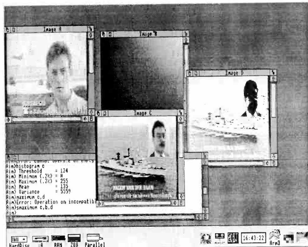
Fig. 5. Linked to !AIM, the digitizer podule and the associated software turn the Archimedes into a near-professional image processing system.
