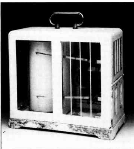
Fig. 7. Definitely a collector's item, this mechanical temperature recorder puts modern electronics in an interesting perspective.
