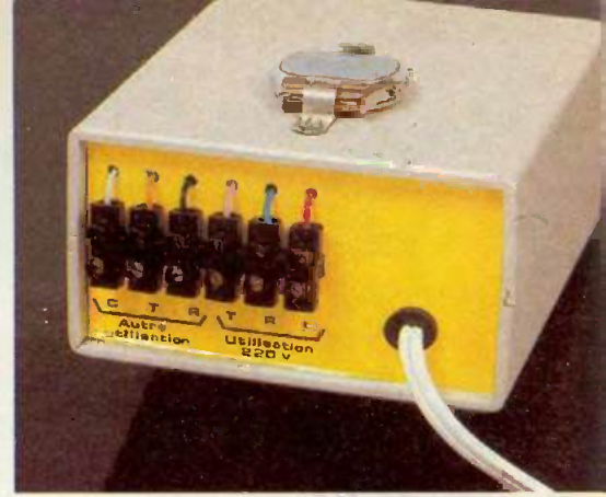
Photo 5. - Dominos de raccordement.
