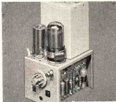
Summing Amplifiers Model 301, illustrated, performs the functions of isolation with low output impedance, as a phase inverter — in conjunction with a network in the grid circuit, as a summing amplifier.
