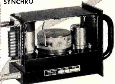
PLUG-IN ASSEMBLIES OF CONTROL MOTOR, GEAR TRAIN, POTENTIOMETER & SYNCHRO
