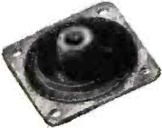
Multiplane Mountings — isolate vibration from all directions. Light in weight, small in size, they are widely used to mount electronic units.
