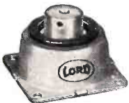
*Temproof Mountings —For Airborne Electronic Equipment • Designed for use with JAN-C-172A cases. • Exceed AN-E-19 drop test requirements. • Maintain efficiency from -80^{\circ} to +250^{\circ} F. *Temperature-proof
