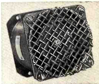
631 x 35 115 Volt, 60 cycle or 220 Volt, 60 cycle, 1 or 3 phase. 3450 RPM continuous duty. 250 CFM at 2 1/2" water gauge. Used in microwave generators; unattended repeater stations. Fits in space 13 1/2" long, 8 3/4" wide, 7 3/4" high.
