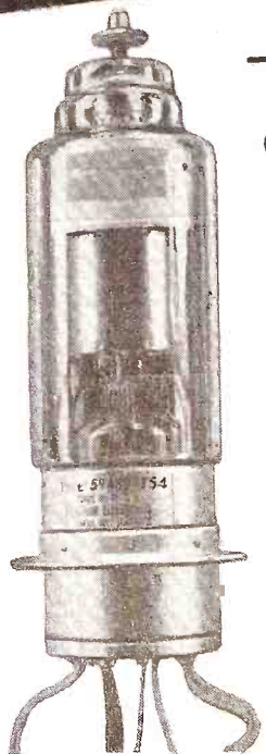
TYPE 5948/1754 Hydrogen filled, zero bias thyatron with hydrogen reservoir for generation of peak pulse power up to 12.5 megawatts.
