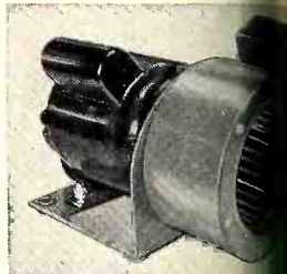
631 x 35 115 Volt, 60 cycle or 220 Volt, 60 cycle, 1 or 3 phase. 3450 RPM continuous duty. 250 CFM at 2 1/2" water gauge. Used in microwave generators; unattended repeater stations. Fits in space 13 1/2" long, 8 3/4" wide, 7 3/4" high.
