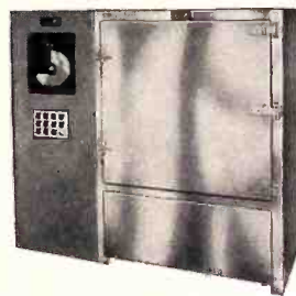
HUMIDITY chamber simulates relative humidity from 20% to 100% between +35^{\circ} F and +200^{\circ} F.
