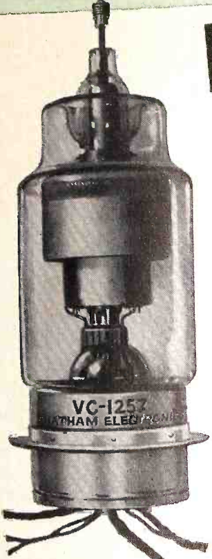
TYPE VC-1257 Hydrogen filled, zero bias thyatron with hydrogen generator for generation of pulse power up to 40 megawatts.
