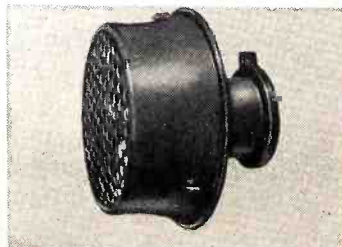
A11A-1—115 Volt 400 cycle single phase propeller type blower using 4" 4 blade fan.
