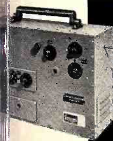
PUNCHED CARD CONVERTER Converts punched data to display point plots.
