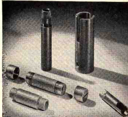
A. Tube, automatic screw machine, turn shoulders, chamfer and thread end, thread other. B. Tube (long pieces), smooth saw, tap threads, screw machine, (small pieces) auto. screw machine, thread, knurl, chamfer, cut off. C. Tube, smooth saw to length, punch twice, countersink. D. Tube, automatic screw machine, chamfer, cut off, punch.
