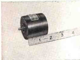
A08C1—2 phase control motor for operation on 60 cycle supply 115 Volt on one phase and 40 Volt on control phase. 3.0 oz/in starting torque on above voltages. 1500 RPM. No load speed.
