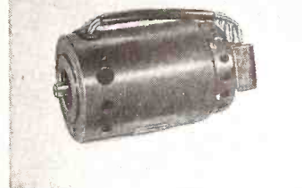
A15HF—115 Volt 60 cycle single phase capacity start & run synchronous motor running at 3600 RPM. This unit has special terminal block mounted on end of motor.
