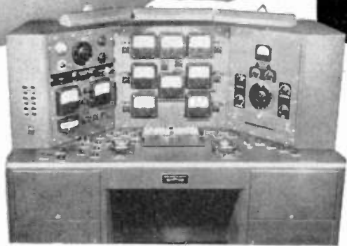
R.F. Universal Power Output Test Set built for Evans Signal Laboratories. Measurements from 20 to 4000 watts; from 2.5 mc to 60 mc.
