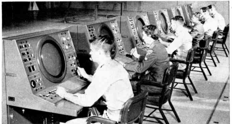
Tracking consoles were put in operation as part of early warning system for Baltimore-Washington area. Du Mont character display tubes show data in the form of letters, numbers and symbols to coordinate Nike missile and other antiaircraft weapons
