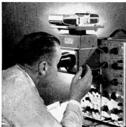
LABORATORY recording of oscilloscope traces is far more efficient with this new camera.
