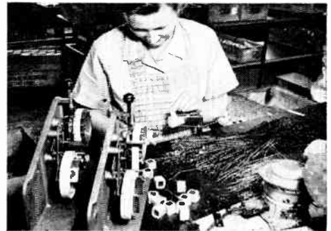
Finish wrap on Woodward-Schumacher transformer coils is made with "SCOTCH" Brand No. 28 acetate cloth tape. Thermosetting adhesive holds tight, giving good conformance and neat appearance. Completed coil is then varnished.
