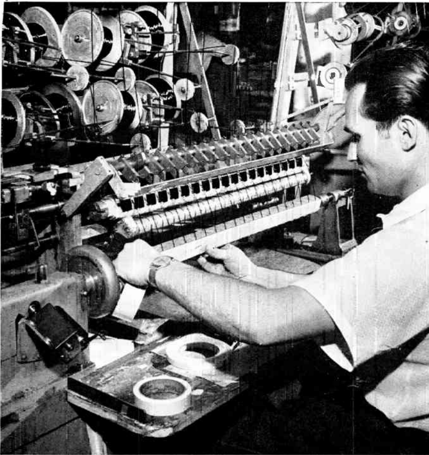
"SCOTCH" Brand No. 39 Tape is used to anchor both start and finish windings. This flatback paper tape has high adhesion, is thin, resists edge tear and is non-corrosive.
