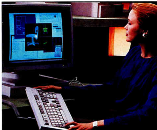
The AV 310c desktop workstation is one of the Aviiion server family, based on SMP architecture.
