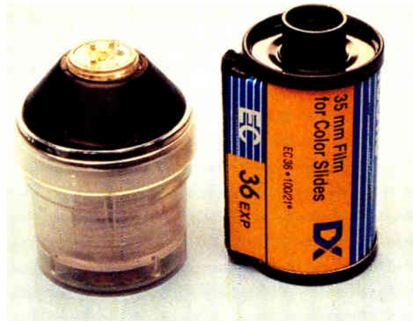
Gyration's mini gyroscope weighs 1.2 oz. and offers real-time response for computer applications.
