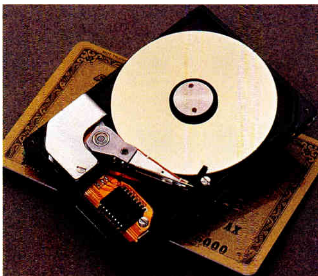
The 1.8-in. hard drives from Integral are small enough for palmtops and rugged enough for some industrial uses.
