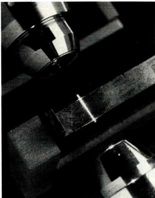
Bellcore researchers are developing an all optical switch that runs at the equivalent of 1 terahertz.
