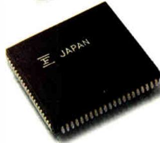
1.5 \mu 3000 Gate CMOS Gate Array
