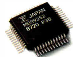
SCSI Protocol Controller with On-Chip Drivers, 48 Pin Plastic Flat Pack
