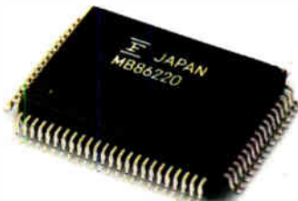
24-bit Floating-Point General Purpose DSP 1.2 \mu CMOS 80 Pin Flat Package
