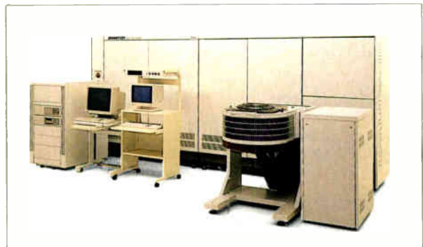
T3344 40/80-MHz, 512 I/O pin VLSI Test System for testing of high-pin count ASICs
