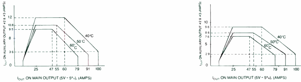
OUTPUT CURRENT ON AUXILIARY OUTPUTS 2 AND 3 VERSUS I_{OUT} ON MAIN OUTPUT (Auxiliary output 4 and maximum output current at appropriate ambient temperature.)
