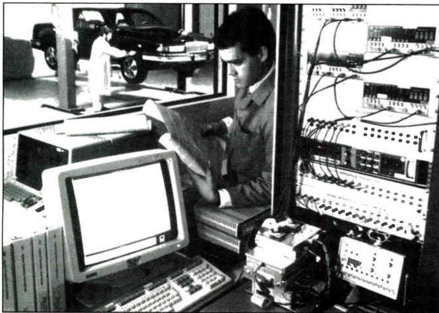
Hughes technician at the GM subsidiary in El Segundo, Calif., operates the firm's Facility for Automotive Simulation and Test to verify Delco design for such systems as antilock brakes.
