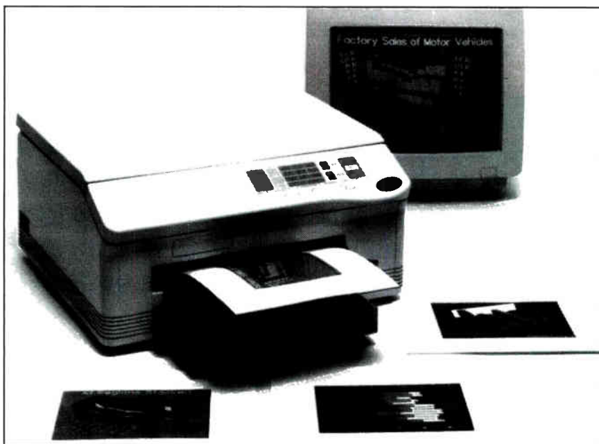
Mitsubishi's G330 color printer pushes thermal-transfer technology to 150 dpi resolution and 4,086 hues while offering a build-in video interface to create faster presentation graphics.
