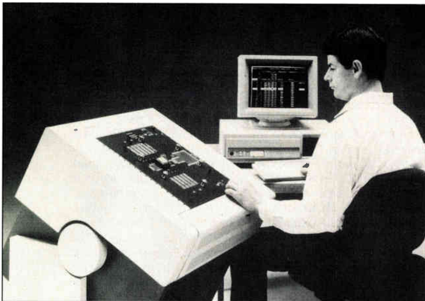
1. SUPERFAST VERIFIER. The Logic Master XL wrings out ASICs at 100-MHz clock and data rates and provides 100-ps timing resolution at each pin with \pm 1 -ns skew.
