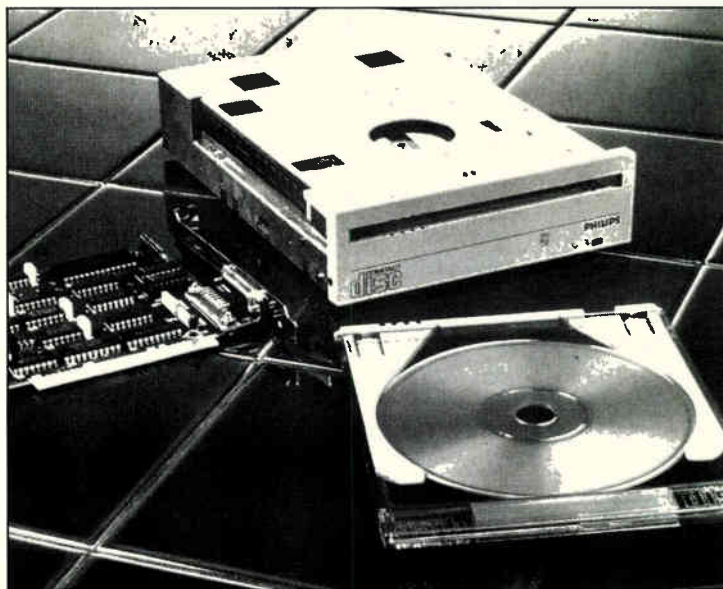
2. ENABLER. Interactive video derived from CD audio will use CD-ROM disks and drives like these made by Laser Magnetic Storage International.
