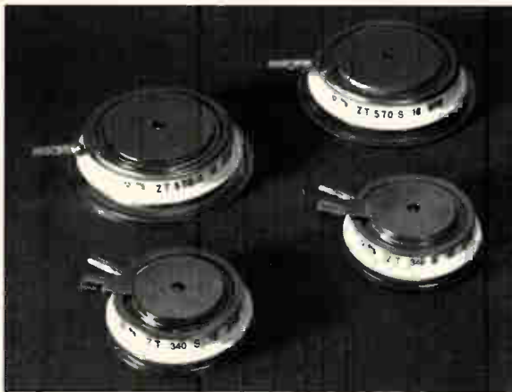
PAIRS. The ZT340s, front, handle peaks of 500 A at 5 KHz and 400 A at 20 KHz, while ZT570s handle 700 A and 900 A.
