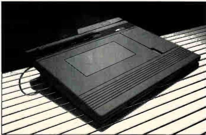
PROGRAMMABLE. Sign/On can tighten pass/fail evaluations for military applications and loosen them for other uses such as retail sales.
