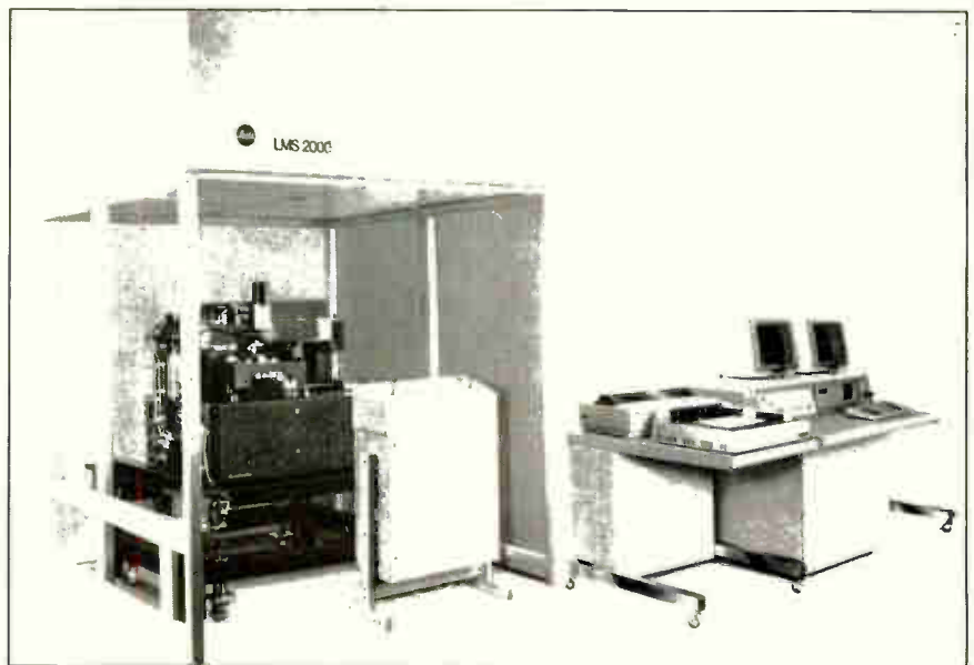
AUTOMATED. Measurements, mask alignment, and focusing on the LMS 2000 are fully automatic, controlled by an IBM Corp. PC AT with a 20-Mbyte hard disk.
