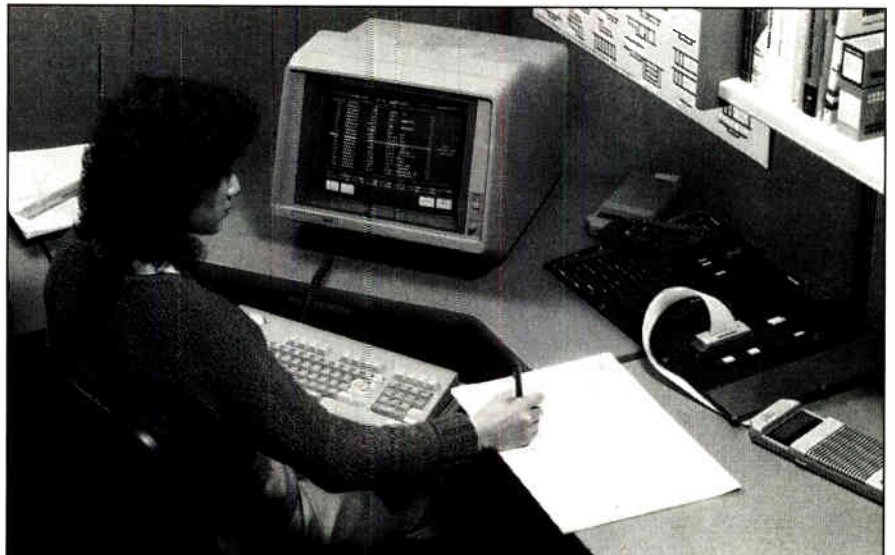
1. MULTIPURPOSE TESTER. Digital analysis systems such as Tektronix' DAS 9200 can replace cascades of logic analyzers for ASIC verification and multiprocessor debugging.
