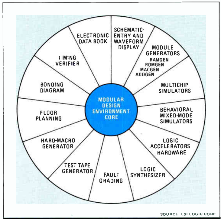
1. TOOL KIT. Supporting the core of the Modular Design Environment are 12 software modules and modified Zycad logic accelerator hardware.
