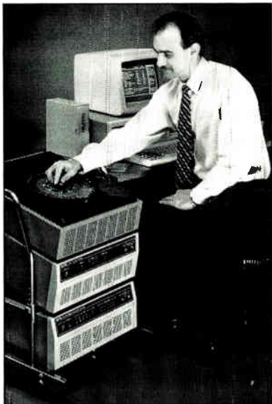
3. DOUBLE DUTY. Hilevel Technology's Topaz ASIC verifier uses simulation software downloaded from the design system.
