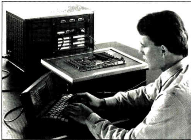
FLEXIBLE. Model 3100 in-circuit tester uses a software-selectable emulation technique and costs only $35,000.
