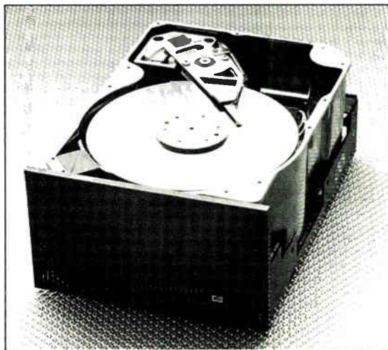
LITTLE BIG DRIVE. Maxtor's latest 5¼-in. drive stores 51 megabytes on each of 15 surfaces and accesses in 18 ms.
