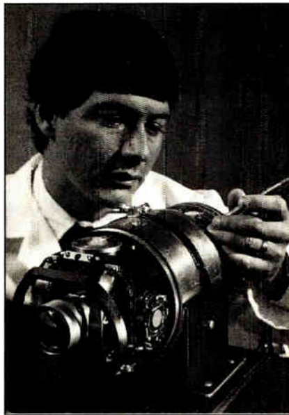
MISSILE EYE. Hughes has delivered IR seekers with PtSi sensors to the Army for tests.
