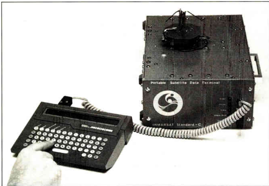
LIGHTWEIGHT. Inmarsat's prototype of a complete data-only marine earth station weighs only 13 lb. Production units should sell for about $5,000 and mount on the ship's superstructure.
