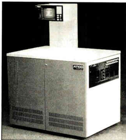
ADAPTABLE. The Smart Power subsystem tests logic and power circuitry together.
